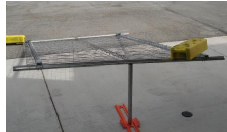
Modified panel 2" deflection under 40# diagonal load.
