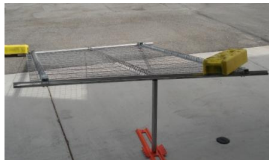
Demo of converted panel 2" deflection under 40# load
